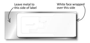
Minimum bending diameter of the Confidex Silverline Classic<sup>TM</sup> is 100mm. For optimal performance please bend the label in the orientation shown below.
